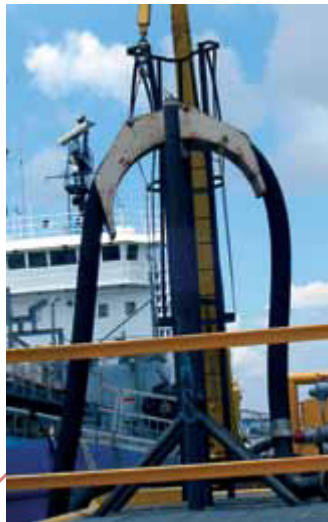
iv. Supporting cradles – custom devices/supports made for a specific application. Hose Cradle Modern Hose Tower Hose Tower
